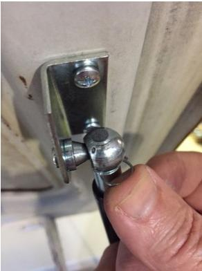
16. Periodically use a non petroleum-based lubricant on the struts and on your trunk gasket so their touching does not become abrasive. <u>Dry</u> Silicone Spray is ideal; available at ACE hardware stores.
