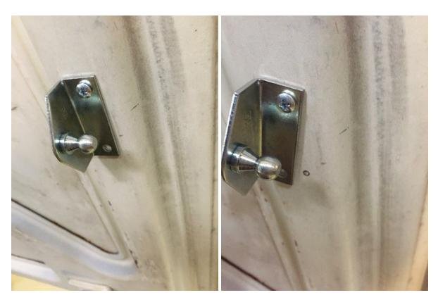
14. Attach the RH gas spring and test operation.
