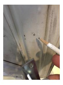
12. Drill this point with a 7/64" drill bit. Note: Use a stop collar on your bit, so you don't accidentally plunge through and dent your boot lid outer surface.
