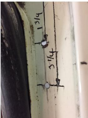
9. Fasten the lower bracket using the machine screws and Kep nuts; see photos. Replace the boot lid gasket.
