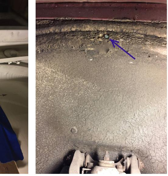
6. Now install the ball stud, using a flat washer and nut on the back side. Hold the front side still with a wrench as shown. Use a drop of thread lock on the nut to make sure it can't vibrate loose.. Note: if you have a thick layer of undercoating, you may have to remove some of it to get the nut fully onto the stud.
