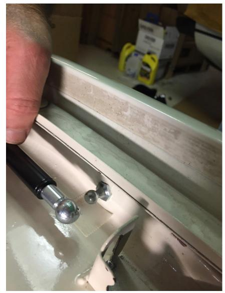
12. Finally, insert the 4 locking wires so the struts are locked onto the ball studs and cannot be knocked off. This can be tricky, because some are blind. It may help to detach one end from its ball stud to insert the first wire (into the other, connected end), and then reattach for the second wire.
