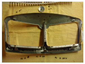
Photo #5, Vane Assembly Removed
